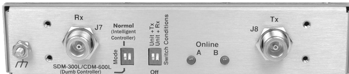
Figure 3-4. CRS-170A – Antenna Side Connectors and Ground Stud (Rev. A and Later Versions)
